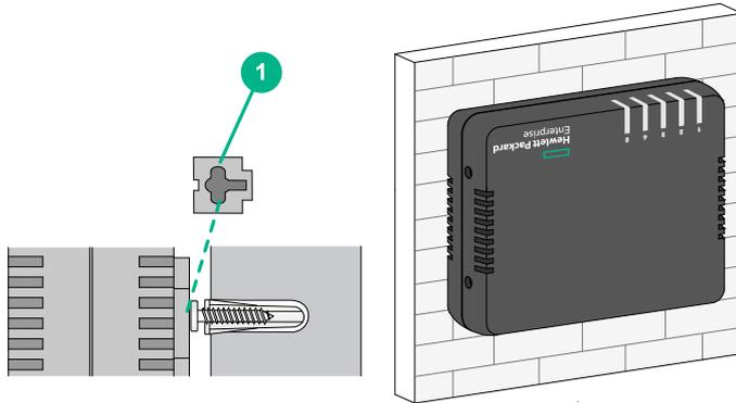
(1) Mounting hole in the switch chassis bottom
