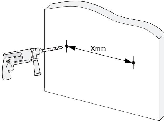
The hole depth and diameter depend on the wall anchors and screws you use. Make sure you can push the anchors to their full depth in the holes.
